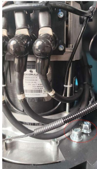
3) Remove the screw and take off the motor power cord connector
