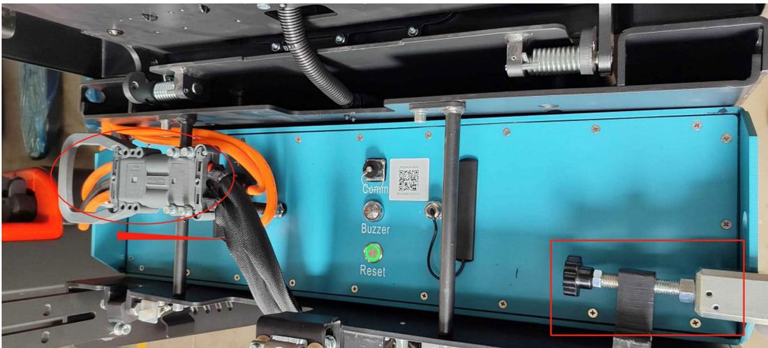
Replace the lithium battery in the same way as the preceding method. Lift the cover, power off, remove the battery discharge port connector, loosen the battery fixing block, and move the battery in the direction of the arrow to remove the battery.
