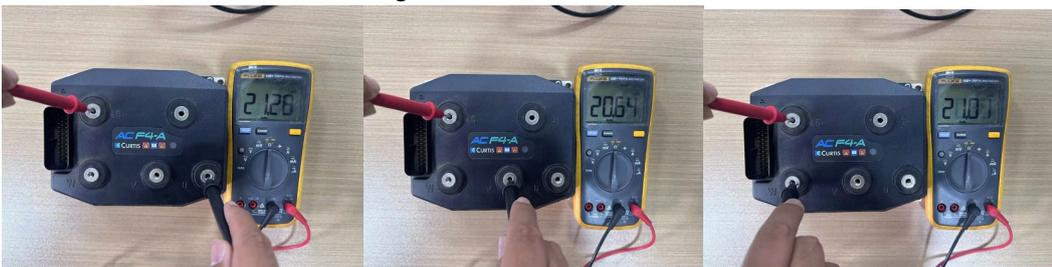
Test 2: measure the diode voltage to u, V and W with red lead, and B + with black lead.
