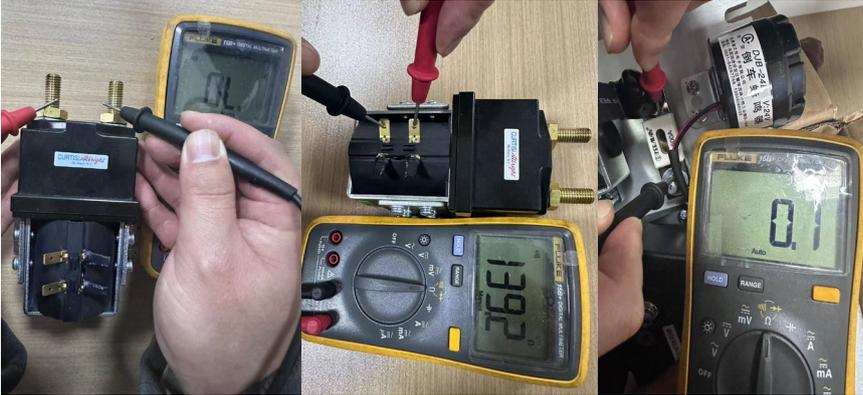
For line contactors and line fuses, connect an ohmmeter (multi meter set to Ohm) at the point shown in the figure and check that it measures the specified value.
