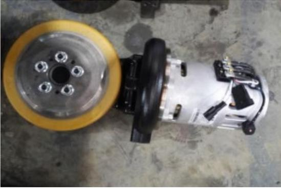
4) Remove and replace the 5 screws fixing the PU ring with a 17mm wrench
