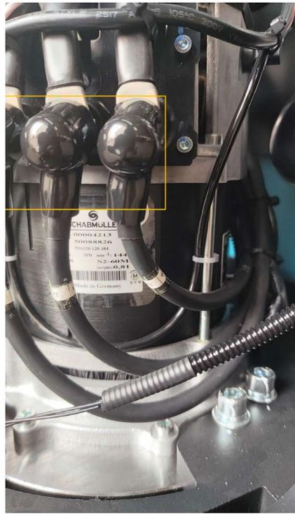
3) Then remove the screws connecting the motor with the car body
